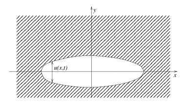
to one variable (say z) and symmetric with respect to another direction (say y). The fracture can then be entirely described by its opening u(x,t) in the y direction (see Figure 2). Since it assumes that the fracture is an infinite strip whose cross-sections are in a state of plane strain, this model is only applicable to rectangular planar fracture with large aspect ratio.
