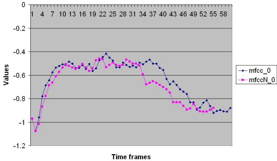
Figure 3.12: Example of time warped template - the variation in time of the first coefficient; the blue dots belong to the original template, while the pink dots to the normalized template.
