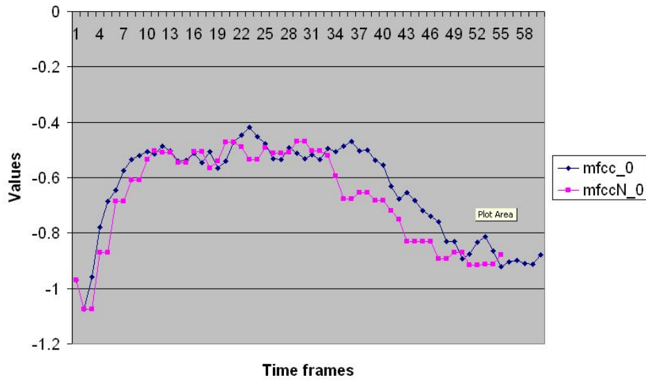
Figure 3.11: Example of time warped template - the variation in time of the first coefficient; the blue dots belong to the original template, while the pink dots to the normalized template.
