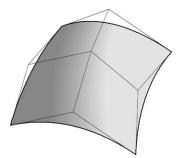
Figure 9.7 A Bézier surface and its control polyhedron
